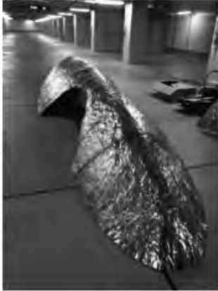
Fig 9. Copper Shell for "Earth: Material for Design" by National Museum of Emerging Science and Innovation. We calculated energy consumption of processing the copper shell by hammering. We found it was only 7 % of the energy used for processing when 93 % for manufacturing copper plate industrially. Design : Jun Sato Laboratory.
